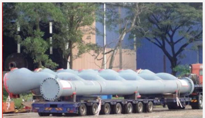
Completed Header Preparing for Shipment
