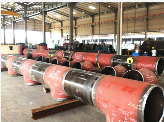
Header Assemblies in Fabrication
